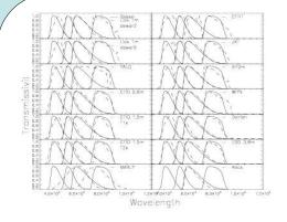
Pass bands are obtained by multiplying filter transmissivity, CCD QE, mirror reflectivity and atmospheric extinction for all instruments. Pass bands are adjusted to reproduce synthetic photometry of calibration stars.
